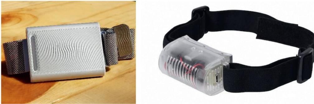
Fig. 6. The Embr TEC bracelet (Embr Labs, Boston, MA, USA) and a commercial TEC forehead cooler.
