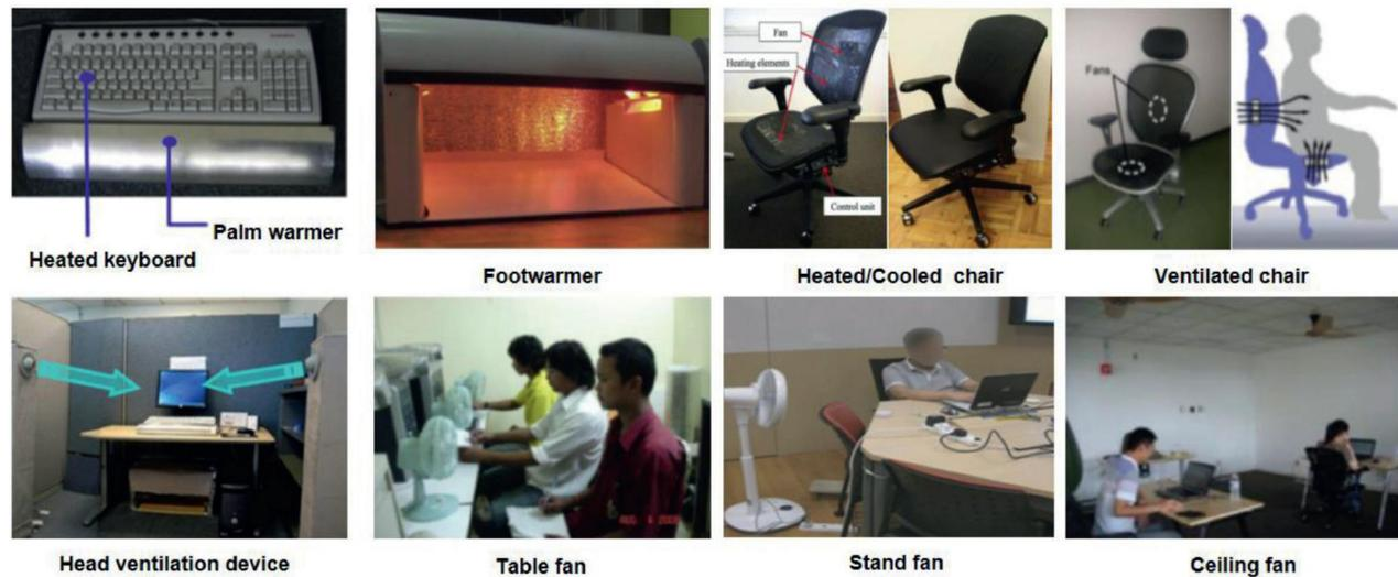
Fig. 4. Different prototypes of PECS (PCS) [55–68].
